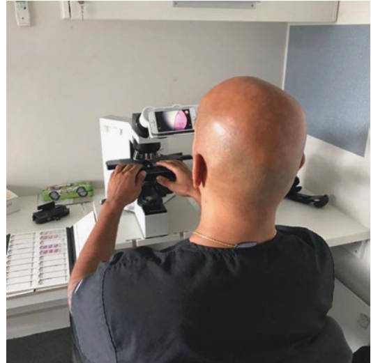
Fig. 17.3 Cheaper systems can be fashioned with a smartphone, teleconference application (e.g., Skype, WhatsApp), and a microscope smartphone adapter (e.g., Labcam, www.ilabcam.com/products/labcam-for-iphone ). This is particularly useful for frozen section assessment of Mohs surgery where the surgeon is able to consult a dermatopathologist at a remote location
