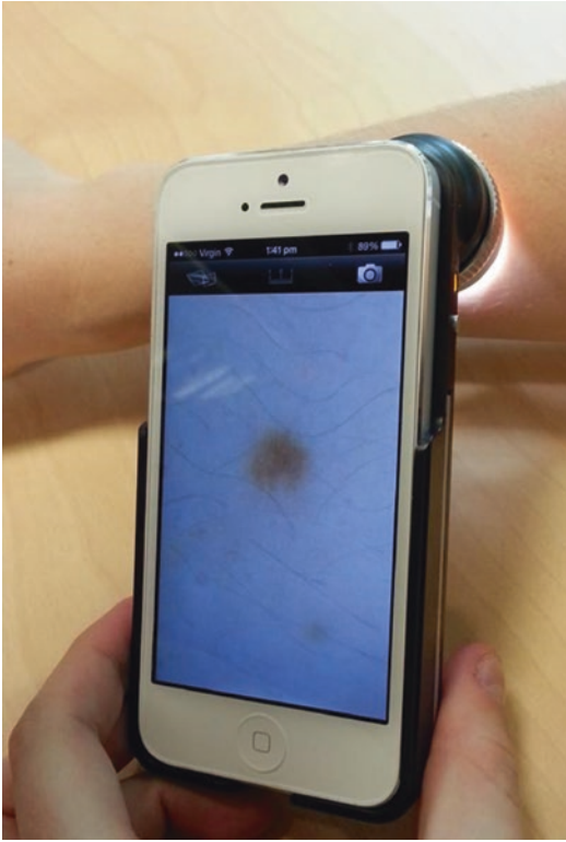
Fig. 16.3 Mobile teledermoscopy utilizes a smartphone with an attachable polarized light dermoscopic lens. Reprinted from “Consumer acceptance of patient-performed mobile teledermoscopy for the early detection of melanoma” by Horsham et al., 2016, British Journal of Dermatology , 175, pg. 1301-1310. Copyright 2016 by John Wiley & Sons, Inc.
