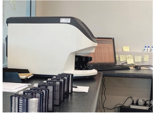
Fig. 17.1 Modern slide scanners have the capacity to scan a huge number of slides daily. This practice has enabled some laboratories to become fully digitalized. Each scanned slide with this system requires the same digital storage space as approximately 1000 MRI scans
