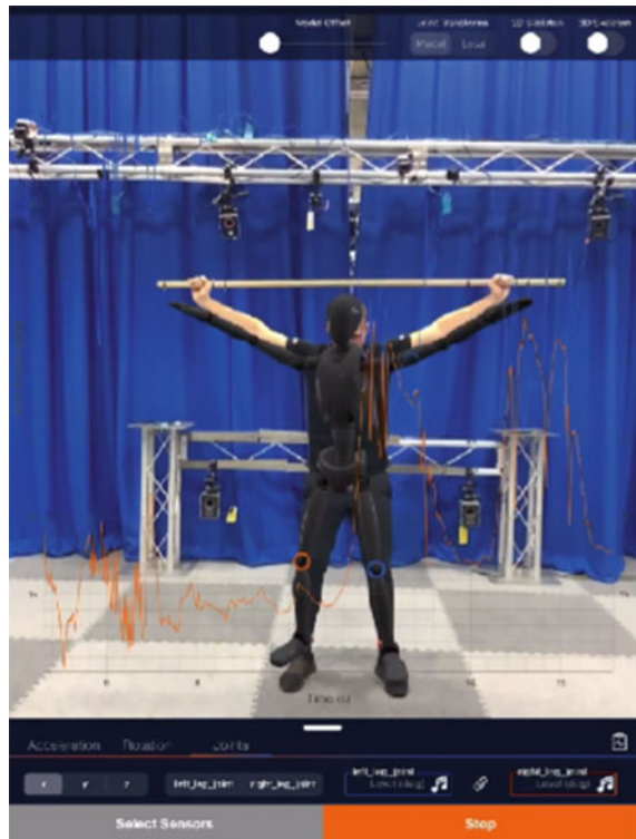
Fig. 14.19 3D model visualisation of squat movements in Capture.U , with a graph of the frequency and amplitude of the movements superimposed on a real-time image (extracted from https://www.youtube.com/watch?v=kRuiol3OqQk )
