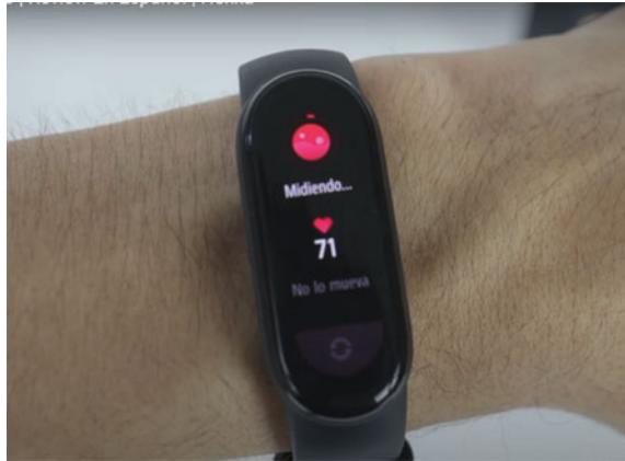
Fig. 14.2 Xiaomi Smart Band 6 performing a blood oxygen saturation (SpO 2 ) analysis (extracted from https://www.youtube.com/watch?v=DiNZT-wL89E&t )
