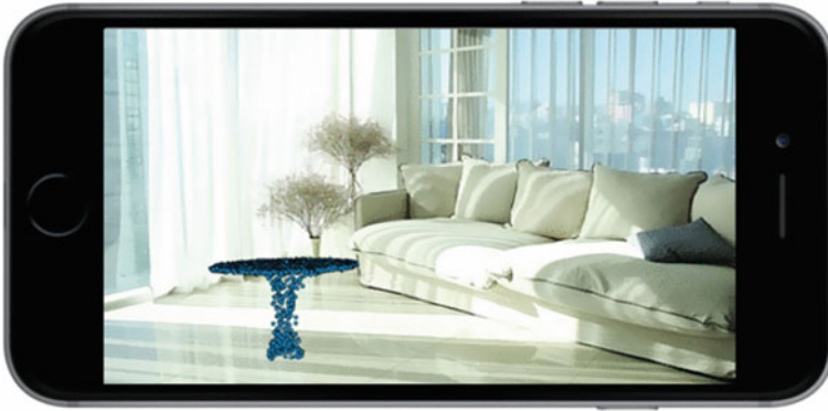
Fig. 1.8 An example of applying a point cloud to an AR application 9 —choosing a piece of furniture to match the surroundings
