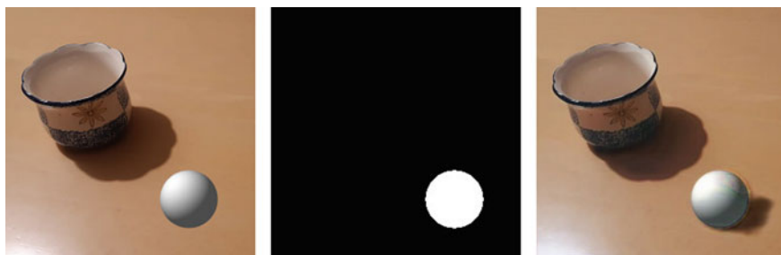
Fig. 1.4 Generating a shadow with ARShadowGAN. 5 Left: the input image contains a real-world background and a computer-generated ball in the foreground. Middle: the mask that depicts the foreground object. Right: the output image with the synthesized shadow
