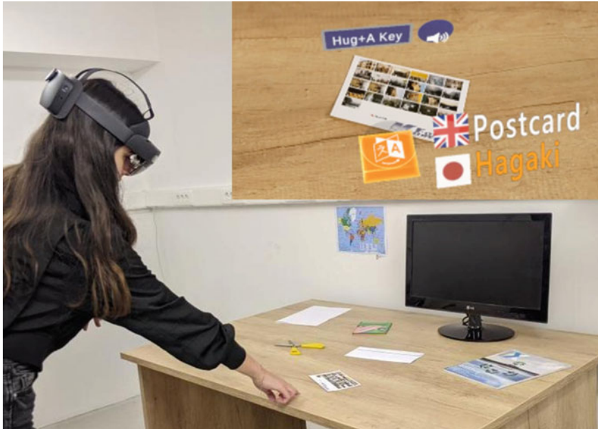
Fig. 16.1 The user is wearing a Head-Mounted Display (HMD) and observing the desk with different objects positioned on it. Utilising object recognition, identification and segmentation the system annotates the scene with virtual buttons. When pressed, the system reveals a keyword together with the English and Japanese words. The system also reads aloud the correct pronunciation of the word in Japanese and shows a memorable link “Hug a key” (Weerasinghe et al. 2022)
