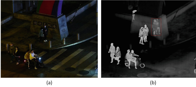
Fig. 1. It can be observed that the illumination conditions are poor and thermal images are more suitable for pedestrian detection than visible images. However, as shown in the red box, the reflection of thermal radiation on the marble surface creates a ghostly image of pedestrians. Adjusting the detector’s propensity for visible or thermal images only based on illumination conditions can easily lead to false detection results. (Color figure online)
