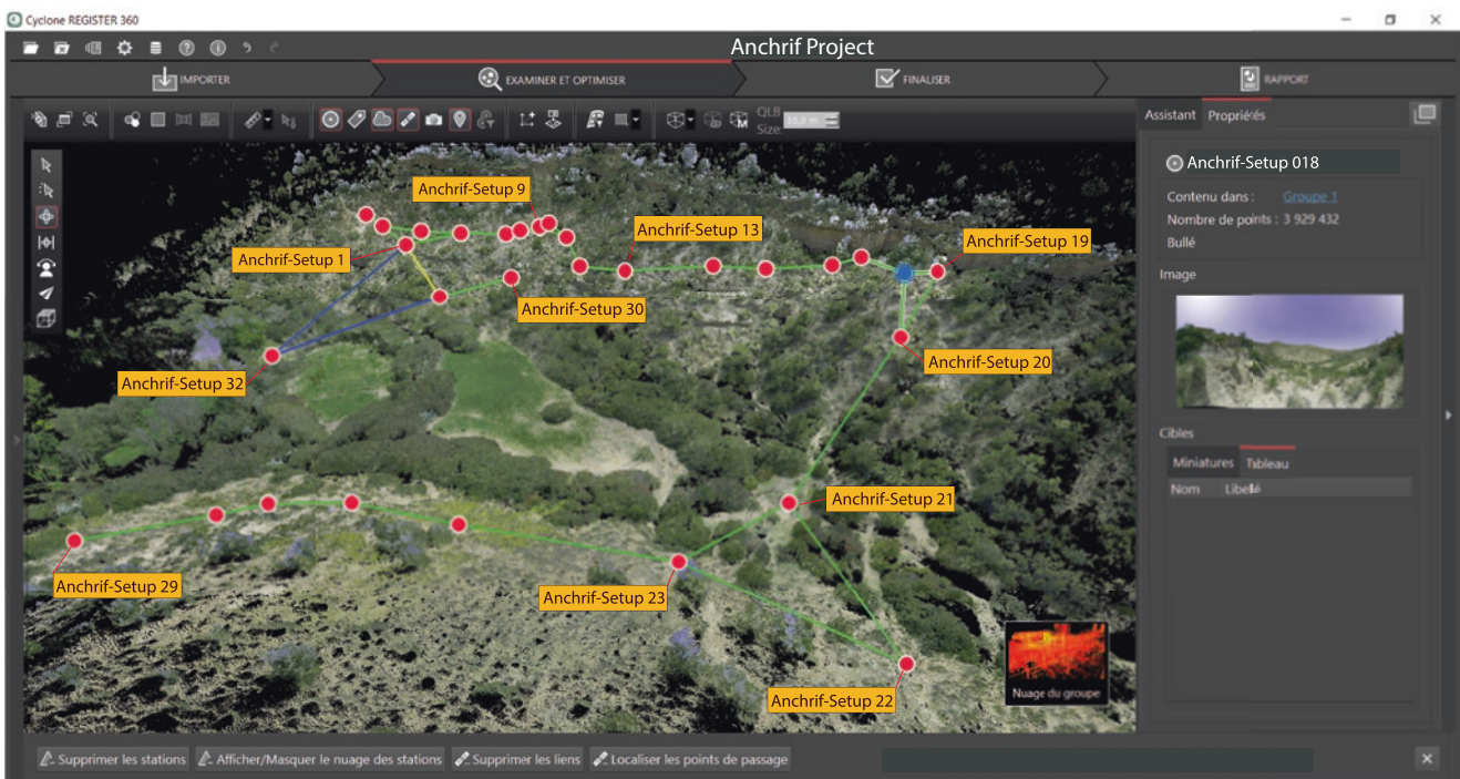
Fig. 7.7 Terrestrial laser scanning of Anchrif site: data preview of survey network and distribution of scanner stations in the import area of Cyclone REGISTER 360
