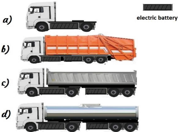
Fig. 6. Other freight possible usages for modular electric trucks: a) electric truck; b) electric trash truck; c) electric dump truck; d) electric tank truck.
