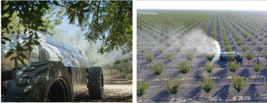
Fig. 8.6 GUSS autonomous orchard mist sprayer
