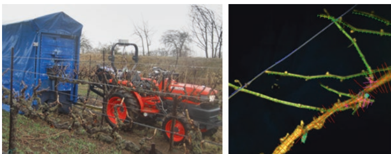
Fig. 8.8 Vision Robotics Grapevine Pruning system towed behind an autonomous tractor (left) and the artificial perception of branches (right)
