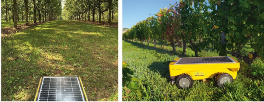
Fig. 8.5 VITIROVER robotic mower fleets can be used to manage grass. This is used to reduce weeds in both orchards (left) and a vineyard (right)
