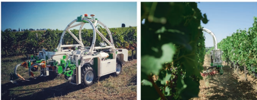
Fig. 8.7 Naïo TED, a mechanical vineyard weeder
