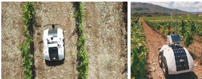
Fig. 8.10 VineScout vineyard monitoring platform
