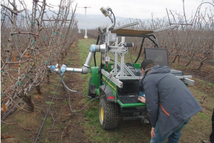
Fig. 6.8 Integrated robotic system for selective pruning of apple and cherry trees developed by researchers at Washington State University and Oregon State University. (Photo by Manoj Karkee)
