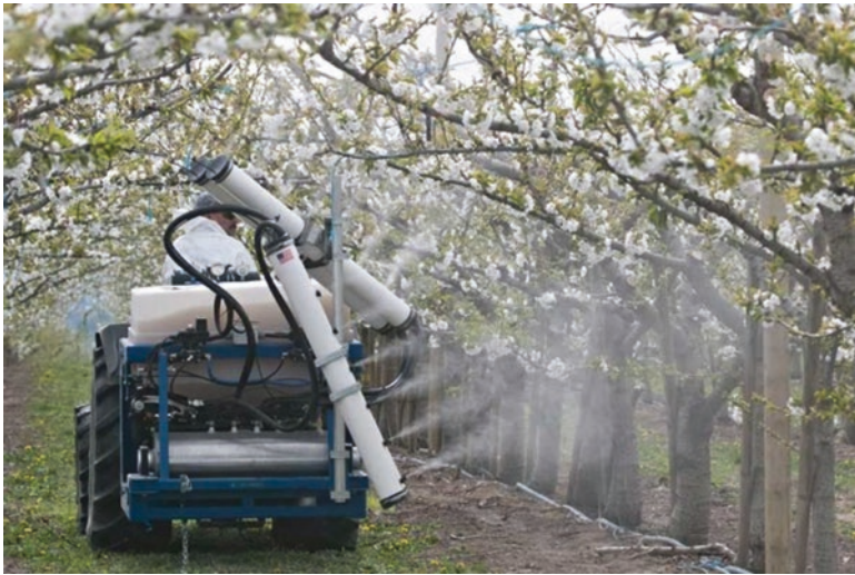
Fig. 6.14 An electrostatic sprayer retrofitted by Dr. Mathew Whiting and his team at Washington State University to apply pollens, being evaluated in a cherry orchard in Prosser, WA. (Picture by TJ Mullinax/Good Fruit Grower)
