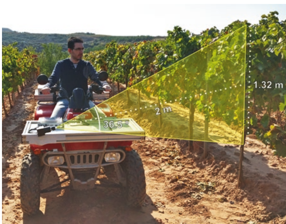
Fig. 5.5 Hyperspectral imaging camera mounted on an all-terrain vehicle moving at 5 km/h used for monitoring a commercial vineyard in Spain. (Photo: Javier Tardaguila)
