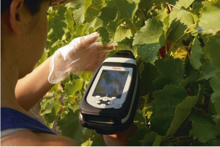
Fig. 4.3 Spectral measurement on the adaxial side of leaves using a handheld NIR (1600–2500 nm) spectrophotometer. (microPHAZIR, Thermo Fisher Scientific)
