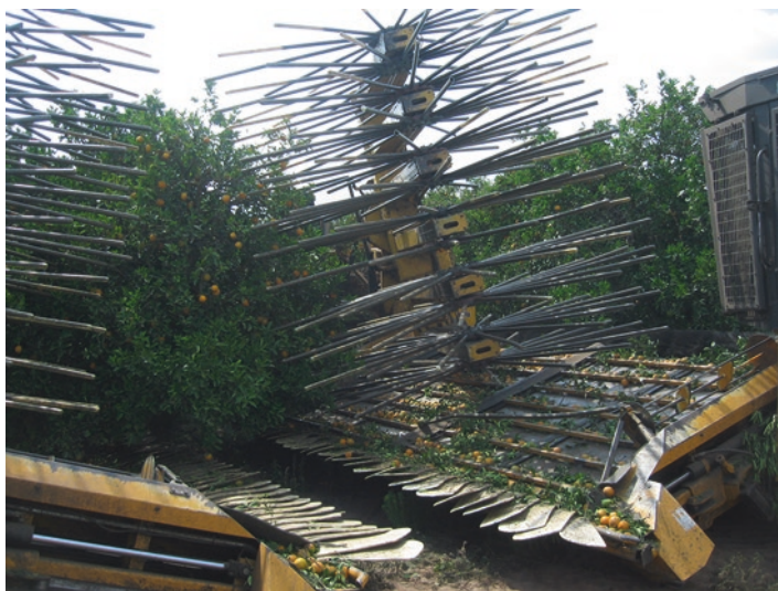
Fig. 7.12 Spindle-based canopy shaking concept of orange harvest system. (Photo by Daniel Guyer)
