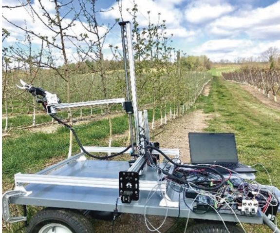
Fig. 2.12 Experimental setup of the integrated pruning system in a Fuji apple orchard. (Zahid et al., 2020b)
