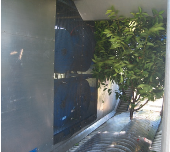
Fig. 7.7 Internal chute of pulsed air blast canopy shaking trial concept. (Photo by Daniel Guyer)
