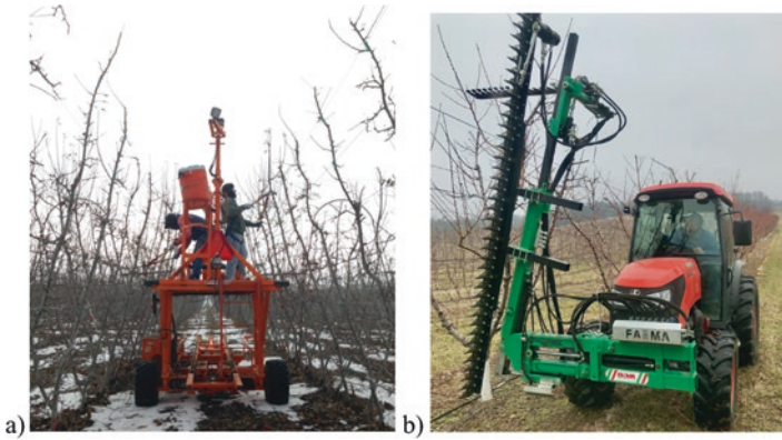
Fig. 2.2 Alternative pruning solutions for tree fruit orchards. (a) Pruning assist platform system (Bandit, Automated Ag) and (b) mechanical hedging system (FAMA hedger)
