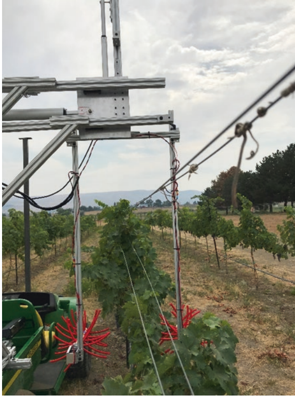
Fig. 6.13 An integrated prototype for automated green shoot thinning in vineyards consisted of a Kinect sensor, platform bed, and thinning manipulator
