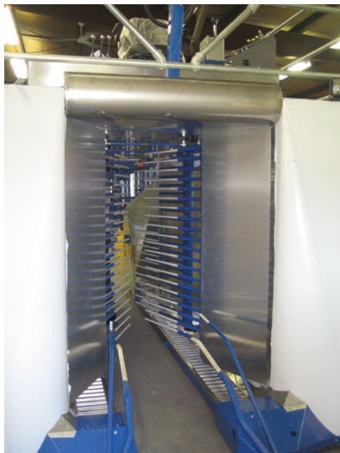
Fig. 7.6 Internal chute of pivot or sway canopy mechanical harvester. (Photo by Daniel Guyer)
