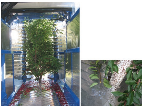
Fig. 7.11 Tree seal "fish scale" fruit catching surface for canopy shakers: (a) showing full shoot and conveyors and (b) close-up of scale engagement with tree. (Photos by Daniel Guyer)
