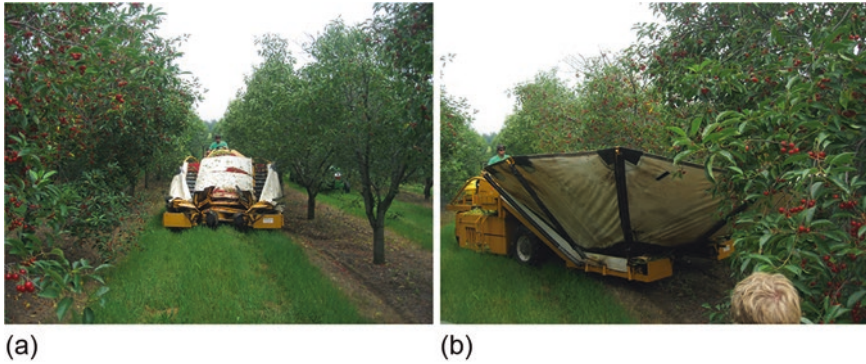
Fig. 7.9 “One-man” harvester: (a) folded moving from tree to tree and (b) in unfolded position during trunk shaking. (Photos by Daniel Guyer).
