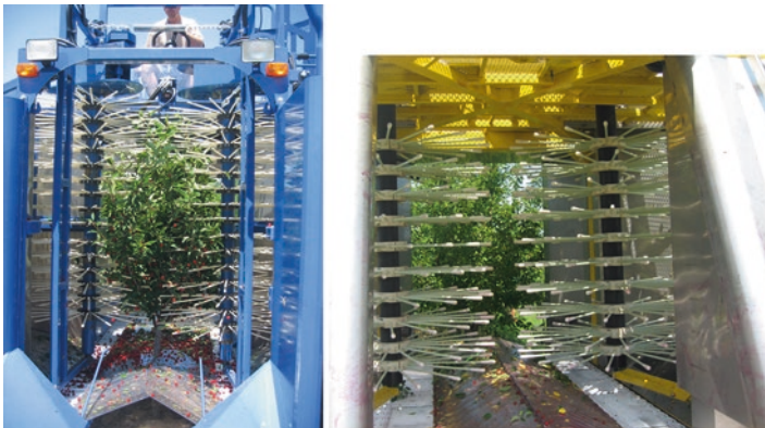
Fig. 7.5 Vertical spindle canopy shaking harvest concepts: (a) commercial blueberry harvester tested on small tart cherry and (b) spindle harvester developed for small trees specifically. (Photos by Daniel Guyer)
