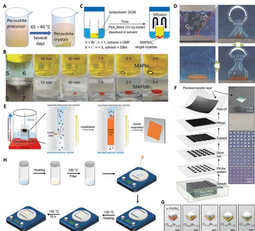
Fig. 3 Solution-based synthesis approaches for both bulk and thin 3D perovskite single crystals. (a) Schematic of solution temperature lowering method. Reproduced with permission from Ref. 60, RSC. (b) Photos recording the growth process of both MAPbI 3 and MAPbBr 3 crystals using inverse temperature crystallization method at different time intervals. Reproduced with permission from Ref. 61, Springer Nature. (c) Schematic of anti-solvent vapor-assisted crystallization method. Reproduced with permission from Ref. 6, AAAS. (d) Schematic of cavitation-triggered asymmetrical method. Reproduced with permission from Ref. 62, Wiley. (e) Schematic of space-confined inverse temperature crystallization method for growing perovskite thin crystals. Reproduced with permission from Ref. 63, ACS. (f) Solution-based lithography-assisted epitaxial growth method and the obtained samples. Reproduced with permission from Ref. 13, Springer Nature. (g) Optical images of the as-grown epitaxial \alpha -FAPbI 3 thin crystals. Reproduced with permission from Ref. 14, Springer Nature. (h) Schematic of space-confined solution epitaxial growth strategy. Reproduced with permission from Ref. 64, ACS
