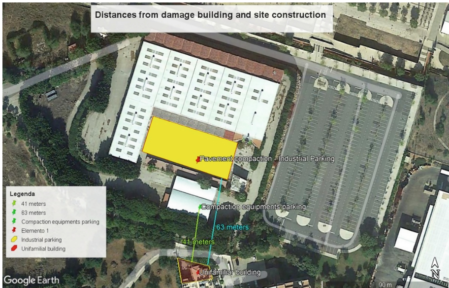
Fig. 1. Distances from the damaged unifamilial building to the industrial park under construction and to the compaction equipment's parking place (Goggle Earth aerial image, taken on February 2020).
