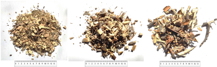
Fig. 2. Resulting product. Blade chipper (left), roller mill: minimum aperture (centre), maximum aperture (right).
