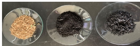
Fig. 2. Aspect of the samples used for this work. CMC raw, Carbonized CMC (100%) and Carbonized CMC+RDF (90–10%).
