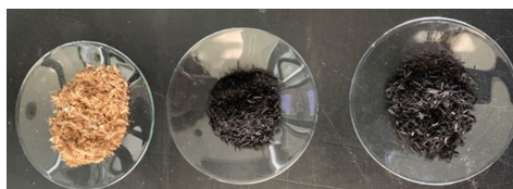
Fig. 1. Aspect of the samples used for this work. OTP raw, Carbonized OTP (100%) and Carbonized OTP+RDF (90–10%).
