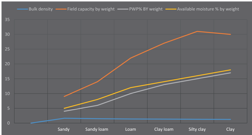
Fig. 2 Soil moisture characteristics of different soils on the basis of their physical analysis (Choudhary 2008)
