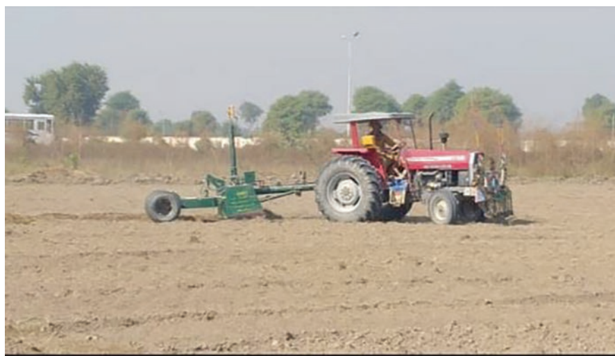
Fig. 7 Laser land levelling at Khwaja Fareed University of Engineering and Information Technology, Rahim Yar Khan
