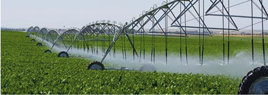
Fig. 6 Central pivot irrigation system
