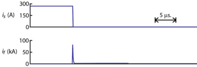
Fig. 7.19 Performance of the flipped \Gamma Z-source breaker during a fault
