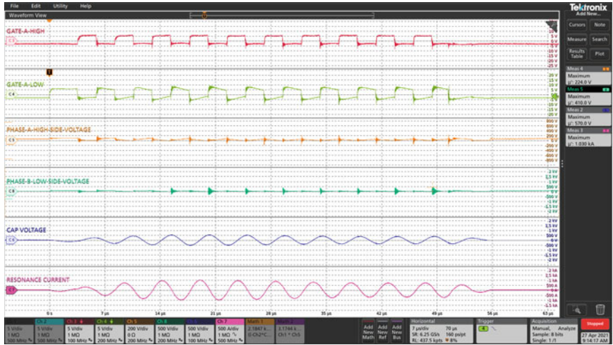
Fig. 14.19 Resonant current-source ramp to 1 kA at 212 kHz
