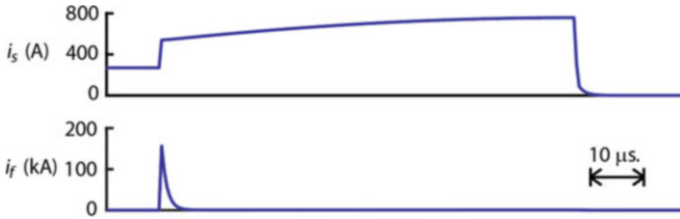
Fig. 7.5 Waveforms of the “parallel” Z-source breaker with in-line components
