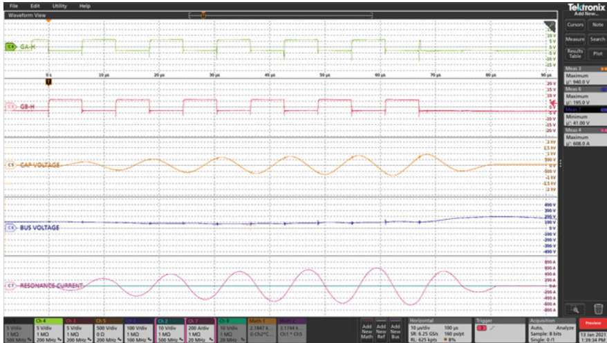
Fig. 14.18 Resonant current-source ramp to 600 A at 82 kHz
