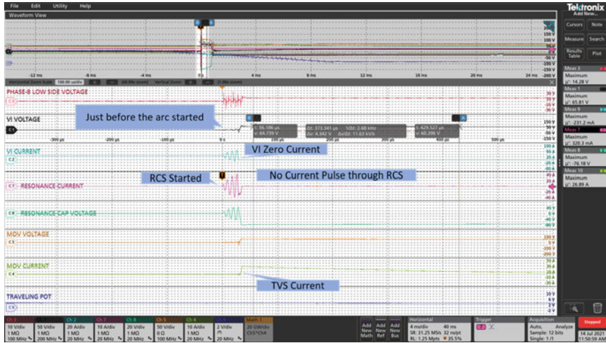
Fig. 14.15 Hybrid resonant DC circuit breaker opening experimental result
