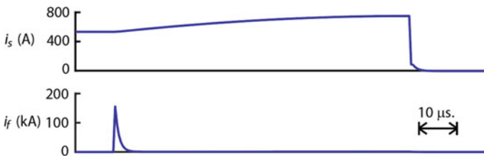
Fig. 7.7 Waveforms of the “series” Z-source breaker topology
