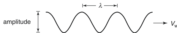
Fig. 1 Properties of a sound wave. All sound waves have a wavelength ( \lambda ), amplitude, and propagation velocity ( v_w ). The frequency ( f ) is inversely proportional to the wavelength
