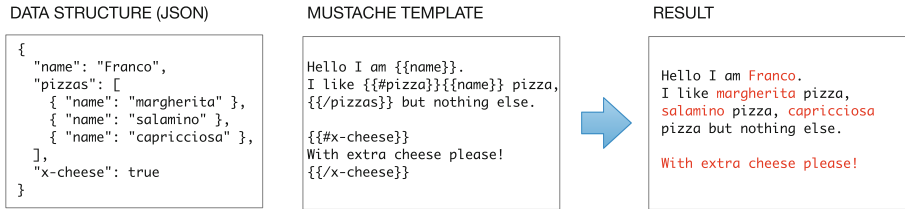
Fig. 1. The data (left) and the mustache template (middle) produce the results to the right.
