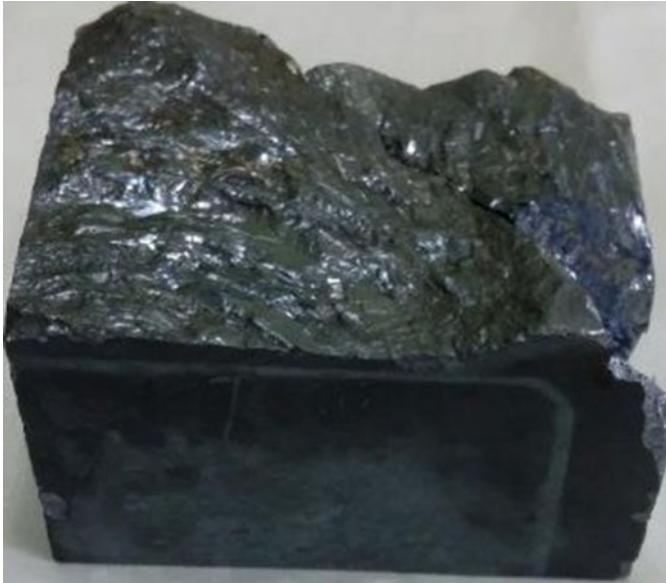
Fig. 2 Ready SCPS ingot in the fault
