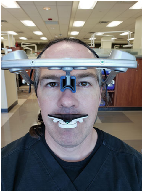
Fig. 5.6 Sensors embedded in the cranial apparatus are used to track sensors located in the mandibular apparatus, which is attached to the patient's teeth
