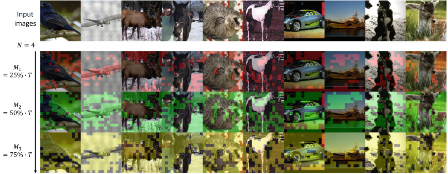
Fig. 2. Visualized examples from STL-10 datasets showing selected patch tokens at the first augmented MSA layer for each sparsity level using the learnt selection.
