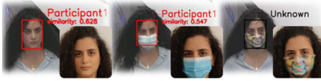
Fig. 1. Illustrating the effect of an adversarial pattern printed on a fabric mask (right), which results in the failure of the FR system to detect the person wearing it, compared to the FR system’s ability to detect the same individual without a mask, as well as with a standard disposable mask.
