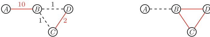
(a) Example for optimal weighted STC. (b) Example for optimal non-weighted STC. The edge weights correspond to the amount of communication. Ignoring the weights leads to three strong edges.
