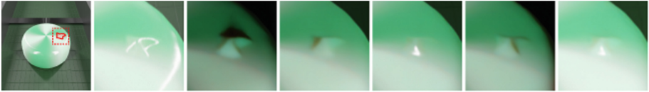
Fig. 3. An anomalous sample from Peppermint Candy category with a bump on its surface. The first figure shows the full picture with the anomalous area highlighted in red. The following figures all show the same crop around the bump, but each one with a different lighting condition.
