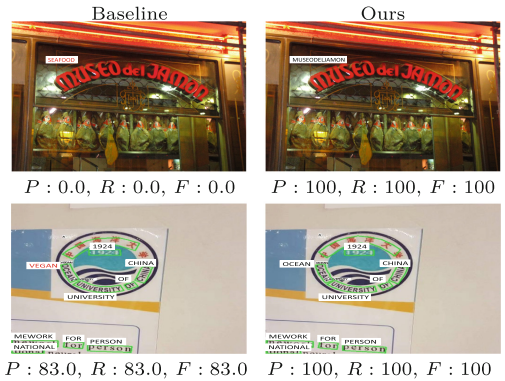
Fig. 5. Text spotting results obtained by the baseline model (left) and our model (right) in Table 3. Detected text instances are marked with green boxes. Incorrect recognition results are shown with red text.
