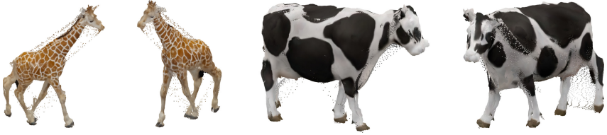
Fig. 4. 3D point cloud reconstruction. The 2D depth estimations from our method can be used to perform 3D reconstruction of the captured shape. The raw 3D point clouds generated by projecting the estimates from all cameras into the common reference frame already yield a good representation. The outliers originate from depth estimates at occlusion boundaries as the L_2 loss encourages smoothed depth maps and could be easily removed by filtering the point cloud.
