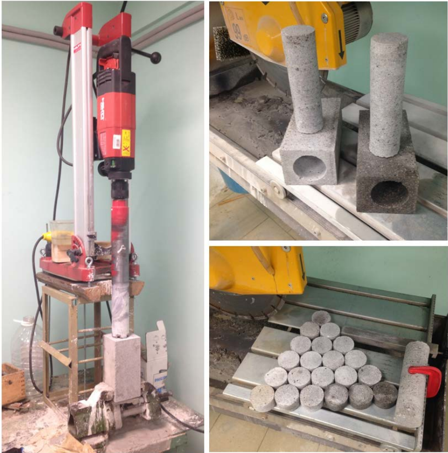
Fig. 18.3: Manufacture of reinforced concrete specimens.
