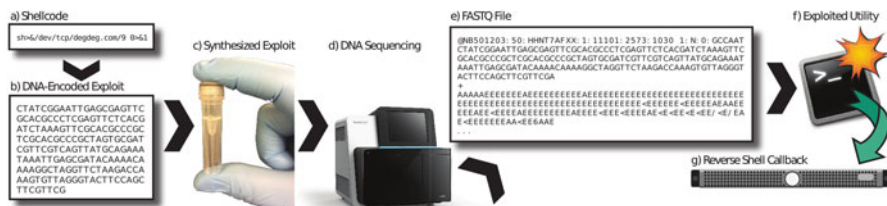
Fig. 1 End-to-end exploit of a computer using DNA. The shellcode was designed, converted into DNA, synthesized, sequenced, and processed by the vulnerable software. After execution, the machine was compromised via a reverse shell
