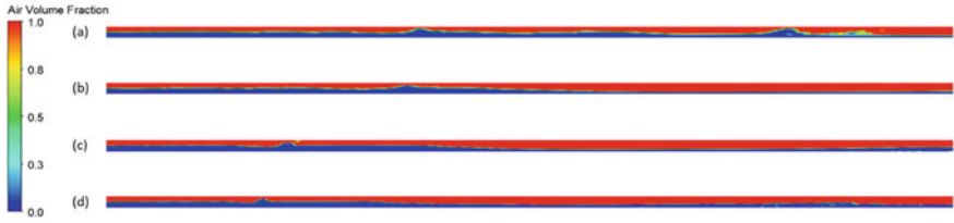
Fig. 5 Results for air volume fraction contours with turbulence damping. Comparison between the onset of slug. Analysis for tridimensional refinement influence. a Coarse mesh (mesh 05); b intermediate mesh (mesh 04); c fine mesh (mesh 06); d extra fine mesh (mesh 07)
