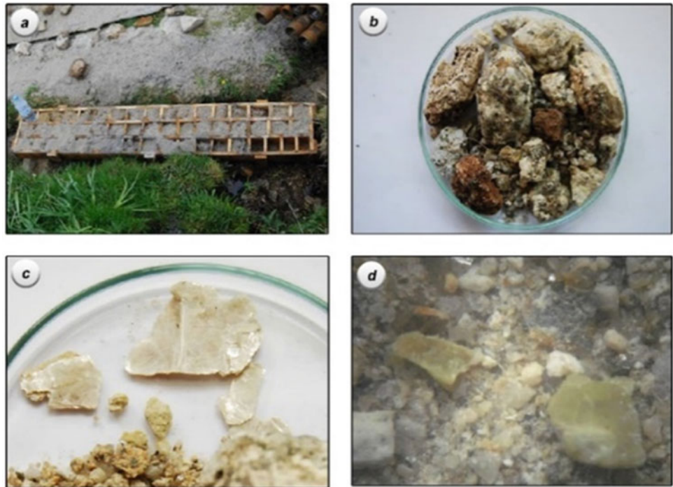
Fig. 3 Field samples in the wooden boxes, collected during drilling (a); Sample from a fractured zone (b); Aspect of some muscovite crystals (c); Portion of chlorite crystals, seen through a binocular microscope with 10 × magnification (d). (Images adapted from Teixeira 2011)
