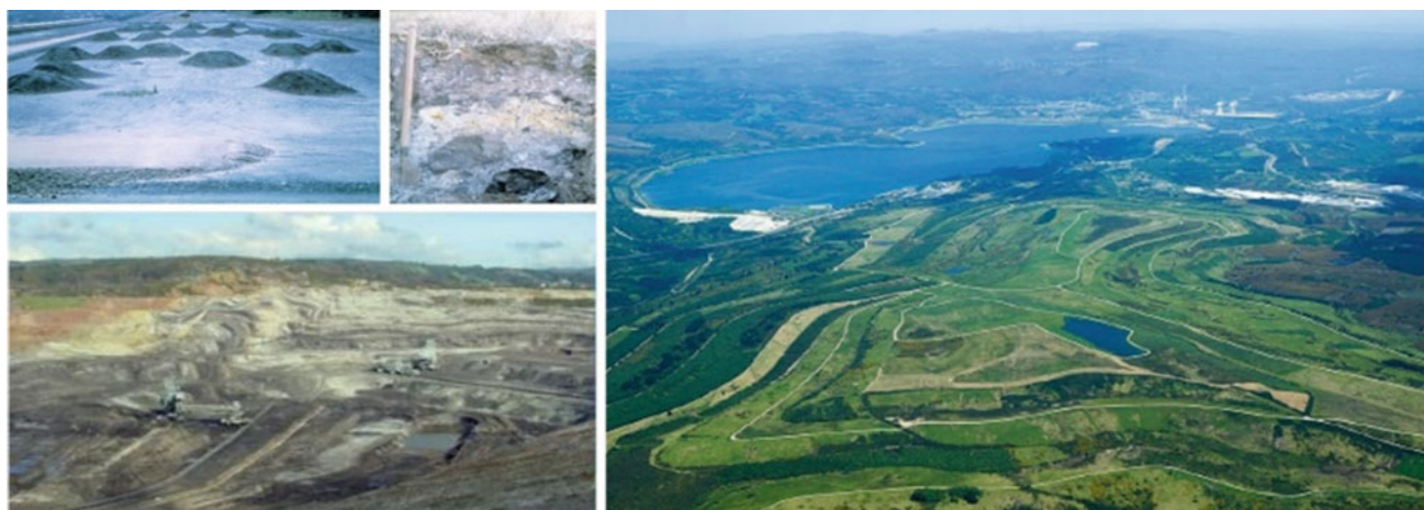
Fig. 1 Recuperation of 1,200 ha of hyperacid, hyper sulphated, heavy metal bearing tailings. Design and EIA of 10 km 2 lake. Rehabilitation of spoiled Technosols and first tailor-made Technosol
