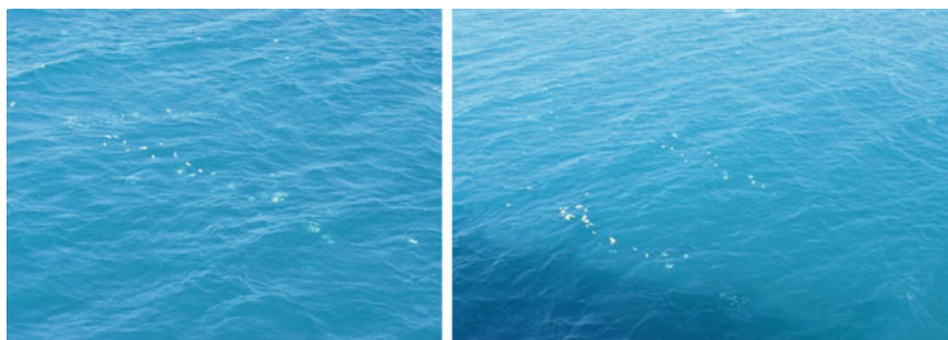
Fig. 5 Visualization of the CL using cut paper markers. Experiment on the oceanographic platform of the Marine Hydrophysical Institute 07/11/2021. Wind speed 17 m/s
