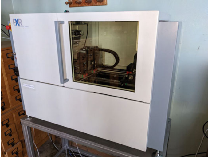
Fig. 1 ProCon X-Ray CT-MINI high-resolution micro-CT scanner of the institute for problems in mechanics RAS
