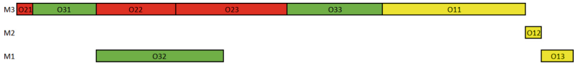
Fig. 5. A revised version of the Gantt chart gained from offline scheduling with the SPT rule.
