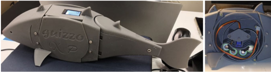
Fig. 15.2 Guizzo Xp: assembly and moving-ballast system
