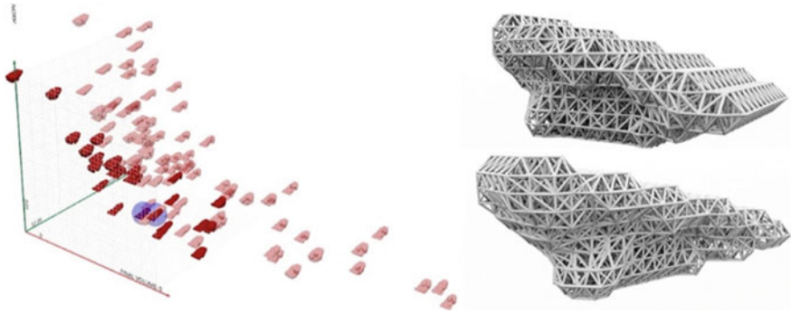
Fig. 17.2 Multi-objective optimization algorithm result for a shoe last design to be produced with additive technologies [11]
