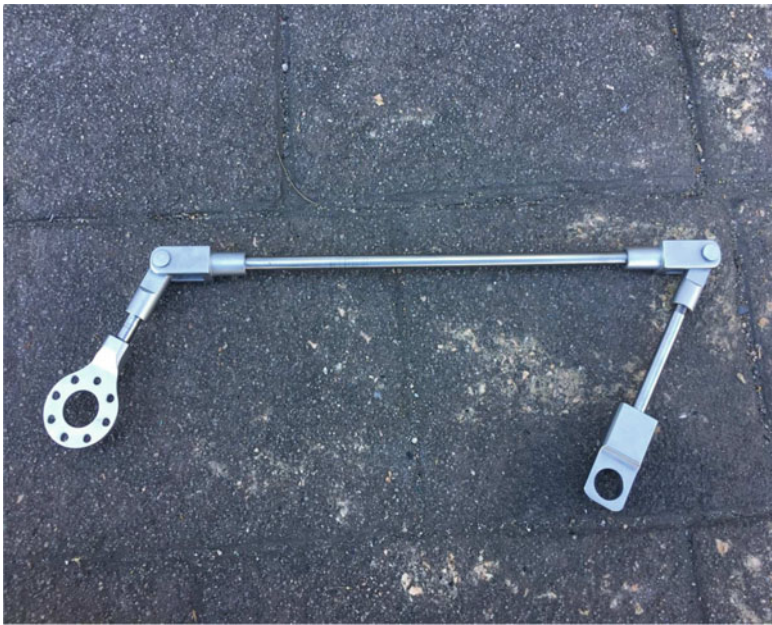
Fig. 8.7 The actual mechanism. Conditions: a smooth motion of the connecting rod b the manufactured mechanism
