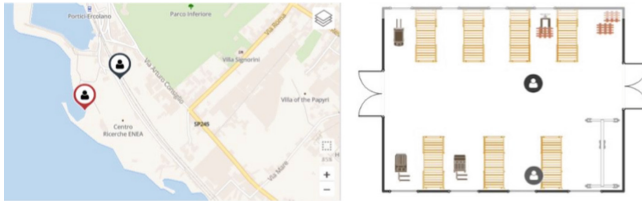
Fig. 3. Dashboard the GPS outdoor position and the RTLS indoor position
