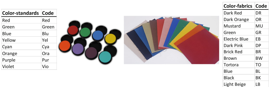
Fig. 1. Test samples: LabSphere® color standards (left) and cloth fabrics (right) – tables of codes.
