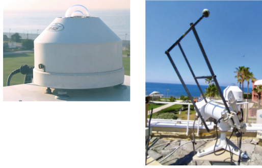
Fig. 2. Solar Tracker with Diffuse Pyranometer, Normal Global Pyranometer EKO mod. MS-802 F and Pyrheliometer HUKSEFLUX DR01-10 (right); Global Horizontal Pyranometer (left).
