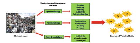
Fig. 10.2 Electronic waste management methods for recovery of valuable metals
