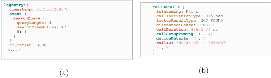
Fig. 6. More examples of Google Dialer ANDROID_DIALER log entries: (a) logging each key press when dialing a phone number, (b) call details sent upon completion of a call, including the call duration (in milliseconds).
