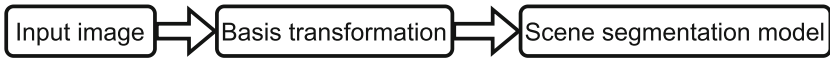
Fig. 2. Workflow of the preprocessing defence. We tested 5 different image transformation functions in the preprocessing layer including JPEG Compression, Bit-depth Reduction, Total Variance Minimization, Low Pass Filter and PCA Denoising.
