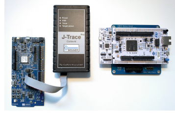
Fig. 2. NRF board connected to the debug and trace probe. STM board on custom break-out board.
