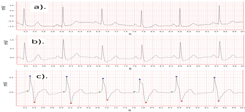
Fig. 2. ECG signals: a) original, b) without baseline wandering, c) without power line interferences but with fiducial points R , S , P .
