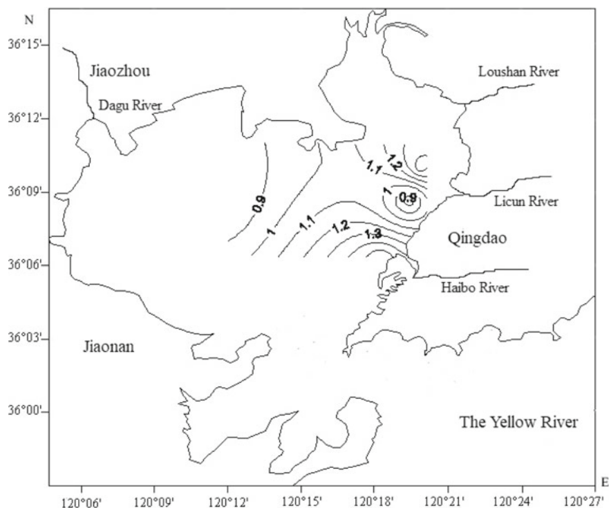
Fig. 87.4 Jiaozhou Bay's Cu content distribution at the surface in October ( \mu\text{g/L} )
