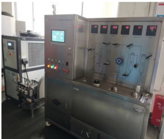
Fig. 43.1 CO 2 supercritical regeneration device
