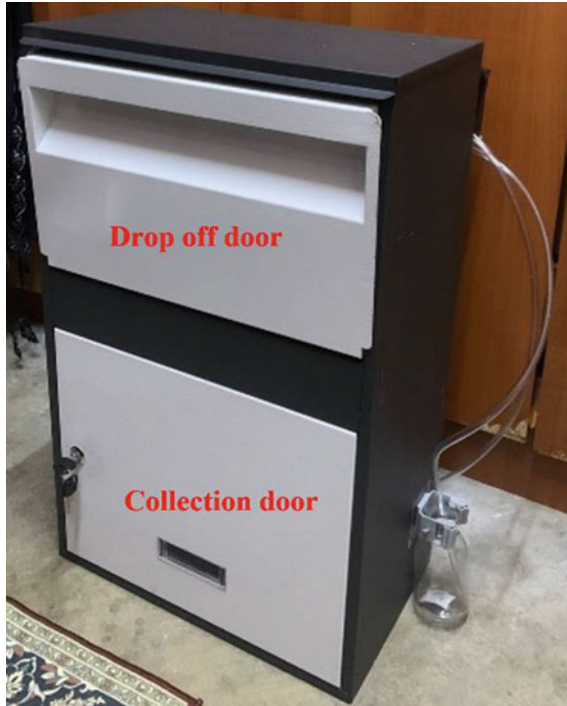
Fig. 6 Smart parcel box with sanitizer prototype
