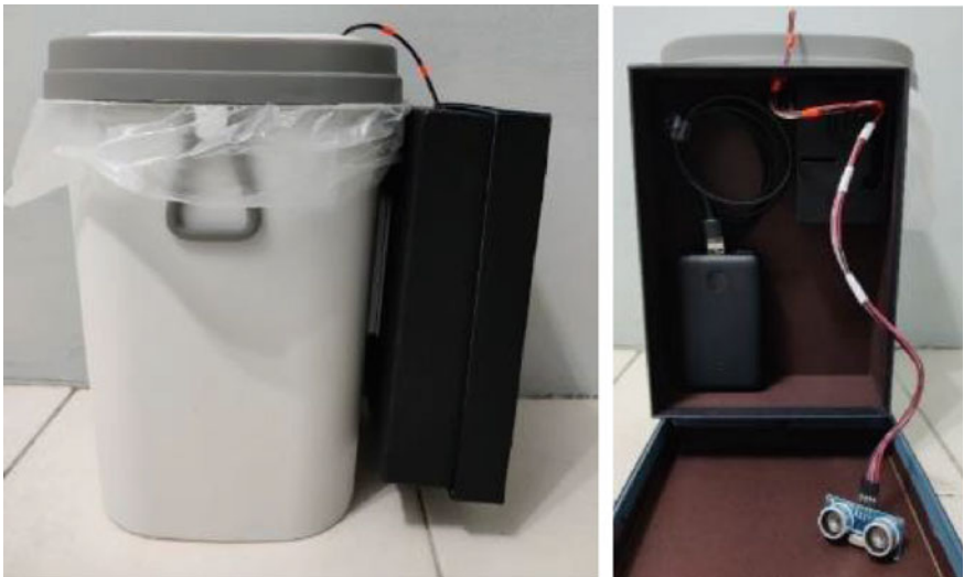
Fig. 5 The prototype for a smart dustbin
