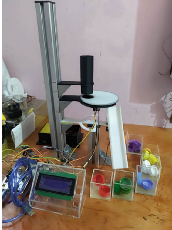
Fig. 4 The fabricated prototype sorts plastic bottle caps according to colors
