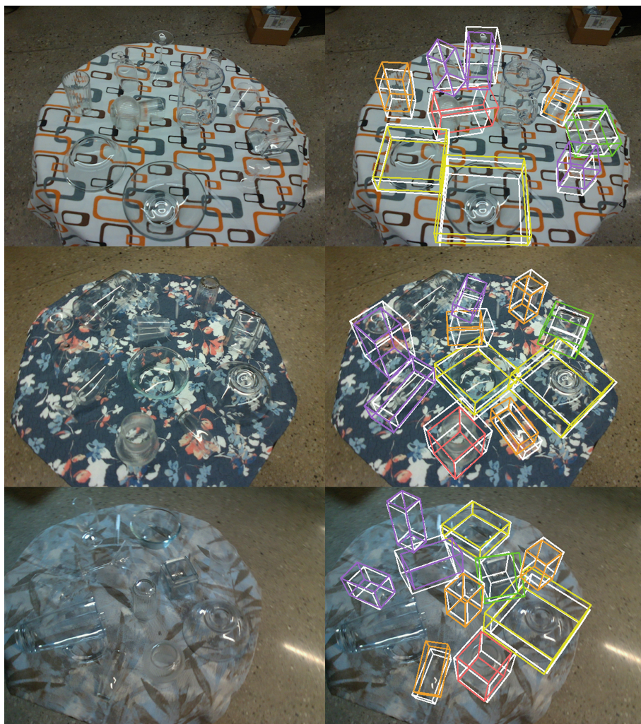
Fig. 4. Qualitative results of category-level pose estimates from TransNet. The left column is the original RGB image within our test set and the right column is the pose estimation results. The white bounding box is the ground truth and the colored one is the estimation result. Different colors represent different categories. For axial symmetric objects, because we only care about the scale and z-axis, we use the ground truth x-axis and estimated z-axis to calculate the estimated x-axis, for better visualization. In the figure, there is a pitcher without either ground truth or estimated bounding box because it is not within any of the defined categories, so we ignore it for both training and testing.
