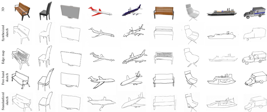
Fig. 3. Synthesized sketches are visually more similar to free-hand sketches than edge maps as they contain distortions and emphasize perceptually significant contours. After standardization, the free-hand sketches share a uniform style similar to training data.
