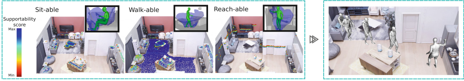
Fig. 4. Action planning as a further step. Left: 3 affordances evaluated in an environment. Right: scores are used to plan concatenated action milestones
