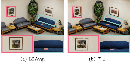
Fig. 5. Initialization comparison. (a) We use PyTorch3D’s rendering pipeline [37] to project each pixel of every RGB image back to the texture. The color of each pixel in the texture is the average of all colors that project to it. This texture minimizes the \mathcal{L}_2 loss of the difference between the rendered and the ground truth images. We dub it L2Avg. (b) \mathcal{T}_{\text{init}} from Sect. 3.1 permits to maintain details. The seam artifacts will be optimized out using TexSmooth (Sect. 3.2). Besides over-smoothness, without taking into account misalignments of geometry and camera poses, L2Avg produces texture that overfits to available views, e.g. , the sofa’s blue colors are painted onto the wall. (Color figure online)
