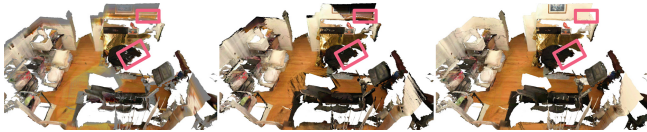
Fig. 11. Results on ScanNet. Left to right: AdvTex-B/C and ours. Ours alleviates artifacts: colors from box on the cabinet are mapped to the backpack and wall.
