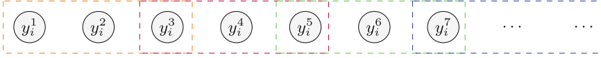
Fig. 7. The 3-ReLU grouping for unstable ReLU neurons in the same layer i , where we use PRIMA to compute the convex relaxation for each group.
