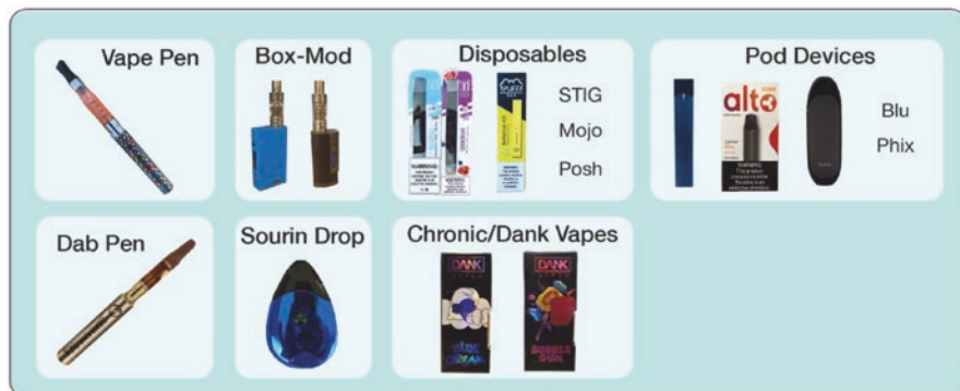
Fig. 7.2 Types of electronic nicotine delivery devices. (Used with permission from E. Hickman, N. Rice and I. Jaspers, UNC Chapel Hill)
