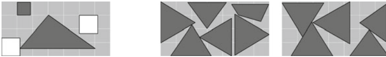
Fig. 62.1 The distance condition (62.2, 62.3) requires that each square of the background grid has to be at least partially covered. Left: a feasible one-bin layout for two tiles (grey) with two support plates (white). Right: an optimal solution using two bins without support plates (instance 3 in Table 62.1)
