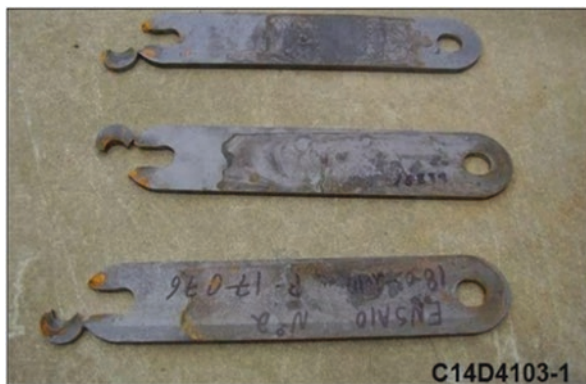
Fig. 19.2 Samples of component C14D41103-1 after the experimental tensile tests
