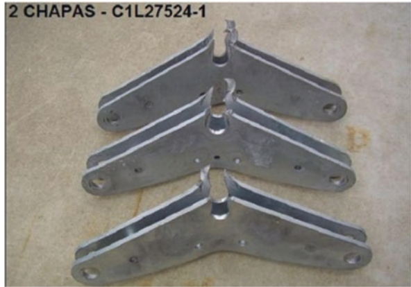
Fig. 19.5 Samples of component C1L27524-1 after the experimental tensile tests
