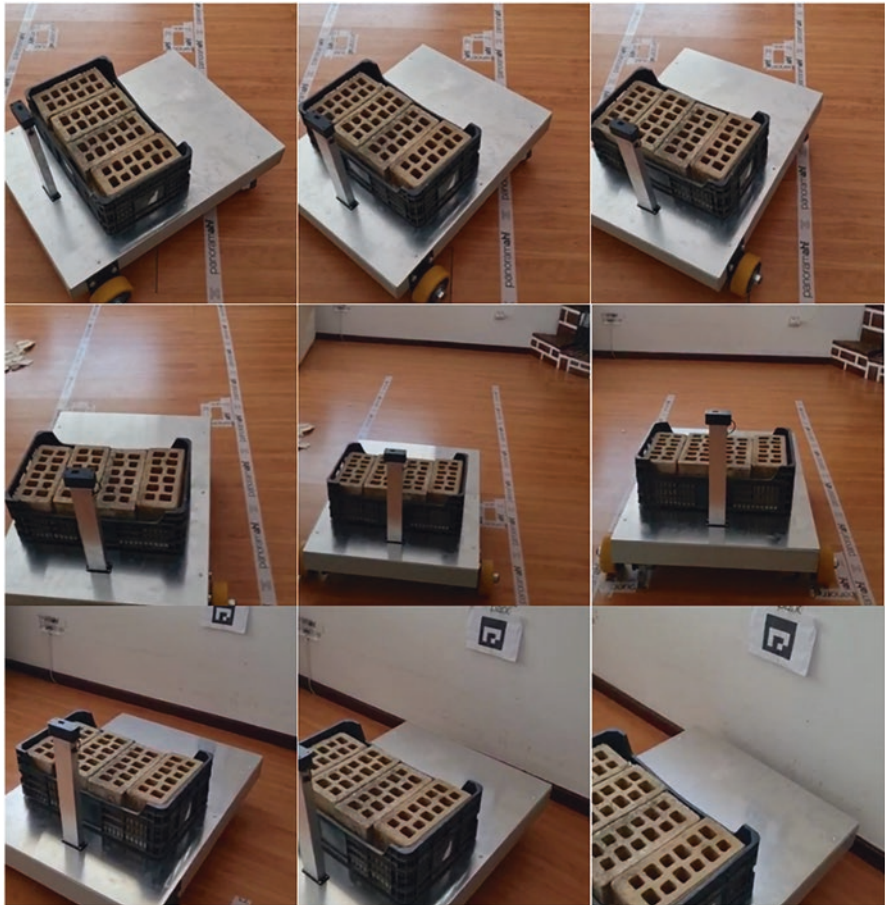
Fig. 20.16 Sequential steps of the AGV searching and approaching the marker (time advancing from left-to-right and top-to-bottom)
