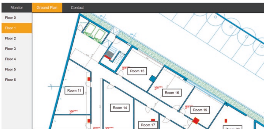
Fig. 5.7 Visualization of one of the software's web interface pages for controlling and monitoring the multiple sensors
