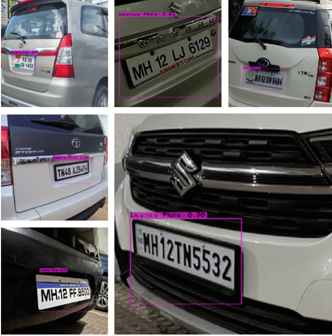
Fig. 3. Examples of detected LP from testing data set
