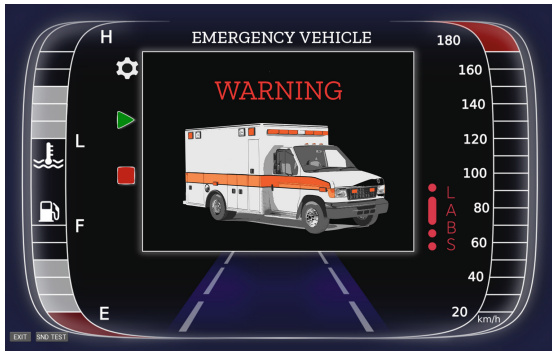
Fig. 5. The HUD GUI showing a car dashboard with a siren alert in the middle.
