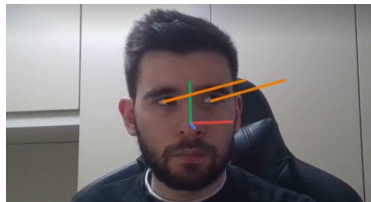
Fig. 7. Gaze Estimation from vision system using a RealSense D455.
