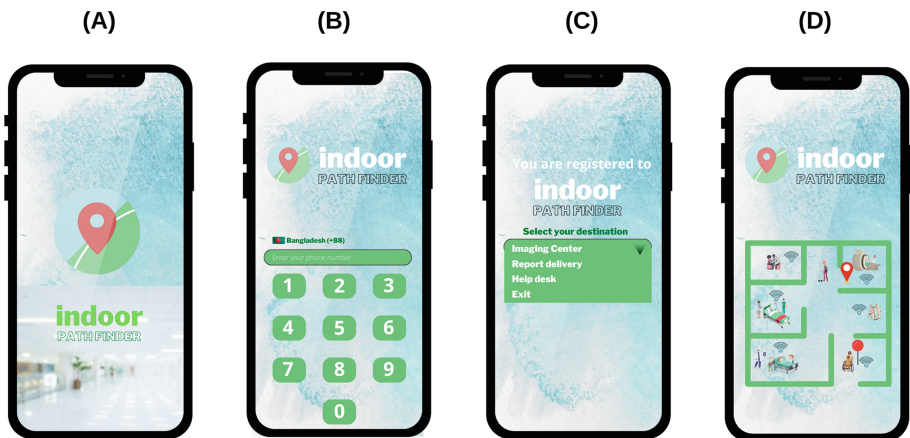
Fig. 9. User Interface for Indoor Navigation: (A) Represents the landing page (B) Shows the app registration with a mobile phone number, (C) reflects the selection of a location using voice command or drop down menu selection, and (D) shows the Indoor Routing Map and placement. The app's compass guides the user to the exact location.
