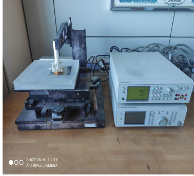
Fig. 2. ECs probe and mechanical automatic scanning device.
