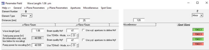
Fig. 6.17 Correction of the beam waist in LASCAD™ Parameter Field by changing the M_x^2 , M_y^2 factors
